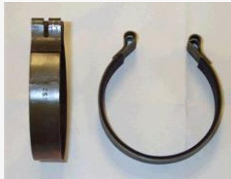
**Flexible lining material bonded on a metal strap,
